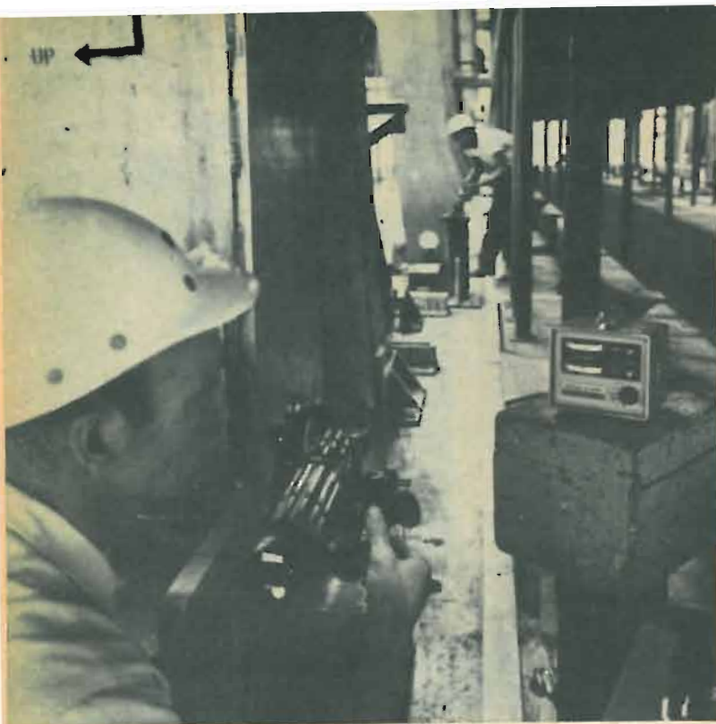
The straight, narrow beam of laser light is used to align tool jigs for the Boeing 747 transport. Accuracy is 0.01" in 200 ft.
